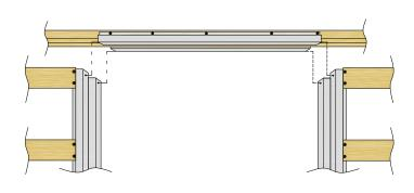
Glass Door Glazing Wedge Elevation View Glazing Wedge Profile Silicone Joint Timber Stud
