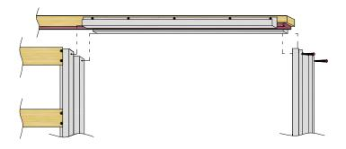
**Detail 13** | **Metinno Aluminium Double Cavity Slider**
