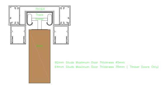
Colour Legends Aluminium Partition (face and section) Steel Stud Plasterboard Profile
