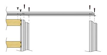
Detail 12 | Metinno Aluminium Cavity Slider with Plasterboard Above
