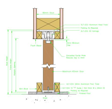
Detail 6 | Metinno Flushline Full Height Detail
