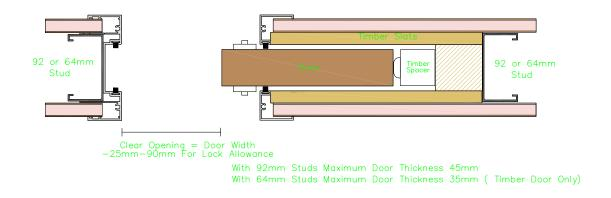
Plan View with Aluminium opening frame. Available for 64mm and 92mm steel studs. Please note only 35 mm doors fit in the 64mm stud profile.
