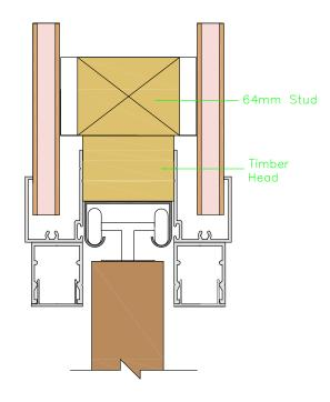
**Detail 19C** | **Metinno Aluminium Receiver to Partition**
