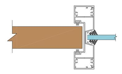
**Detail 19E | Metinno Aluminium Cavity Jamb Detail**
