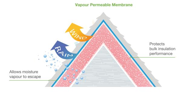
In certain climates and applications, condensation from inside the building may cause a build up of mould and mildew. For these applications, Vapour Permeable Building Membranes act as a water barrier with the additional benefit of allowing moisture vapour to escape from the building.
