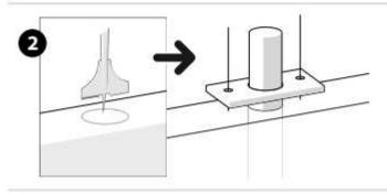
Using a 1 inch spade bit, bore a holde to the depth of 3.75 inches (the length of the release system cylinder). Firmly push the system into the drilled hole and secure with the two screws provided (screws must be counter sunk). Now your door is ready to be fitted. We recommend installing the release system with removable hanger plates or "flip & clip" hardware.
