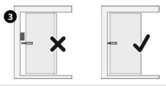
Ensure that there is no object between the back of the door and the back stud inside the pocket, which would prohibit the plunger on the release system from being fully depressed (see diagram). The pocket back stud and back edge of door must be plumb allowing the gap between door and back stud to be parallel.
