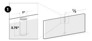
Flush Doors: With the door dismounted, measure and find the centre on the back edge of the door.
