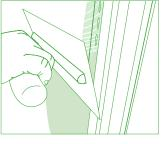
Flush in the set bead frame and sand
