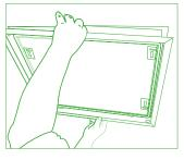
Insert access panel into the cut out
