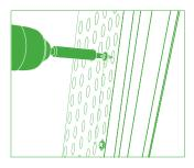
For set bead frames screw through perforated edge
