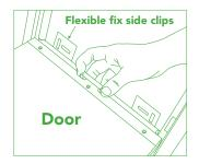
Remove door using the quick release hinges
