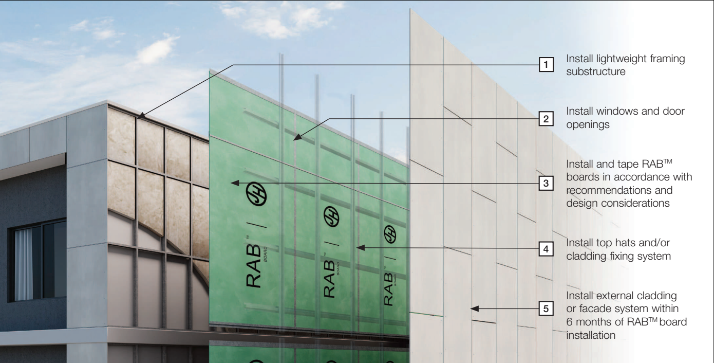
FIGURE 1 OVERVIEW OF THE WALL SYSTEM
