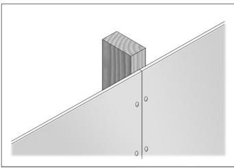
FIGURE 13 SHEET FIXING - BUTT JOINTING
