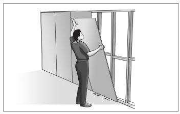
FIGURE 4 SHEET INSTALLATION
