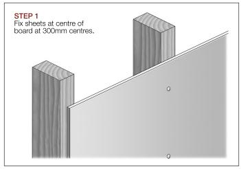
FIGURE 9 STEP 1 - FIX FIRST SHEET
