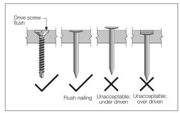
FIGURE 2 FASTENER DEPTH
