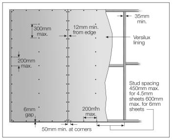
FIGURE 6 WALL FIXING
